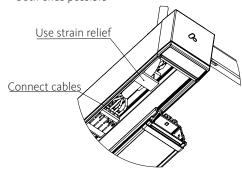
**5:** Mount inner profile Cross section visualization KEEP INSIDE CABLES AWAY when mounting inner profile!
