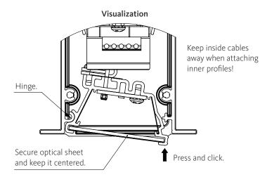
**5 b**: Keep inside cables away when mounting inner profile!
