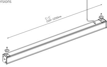
**Installation of ceiling mounts for wire.** Attach the ceiling brackets with screws designed for the current ceiling. C/C 1100-1200 mm. tScrew the wire brackets in the ceiling brackets.
