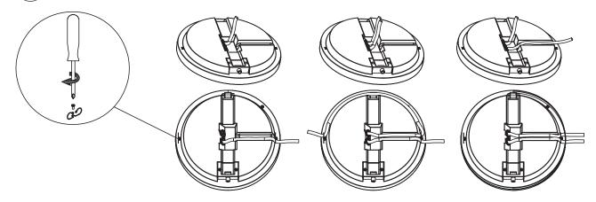
5 Secure the bracket to the ceiling.
