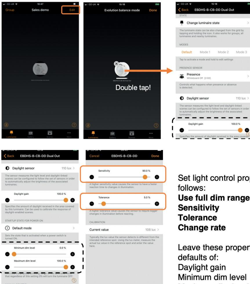
The desired target and light control speed of response is set within the chosen scene as mentioned earlier in the set up steps.
