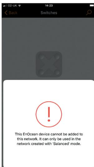
Incompatible units added when in 'better performance' mode networks can fail with this warning. Use 'balanced' mode instead should this message appear.
