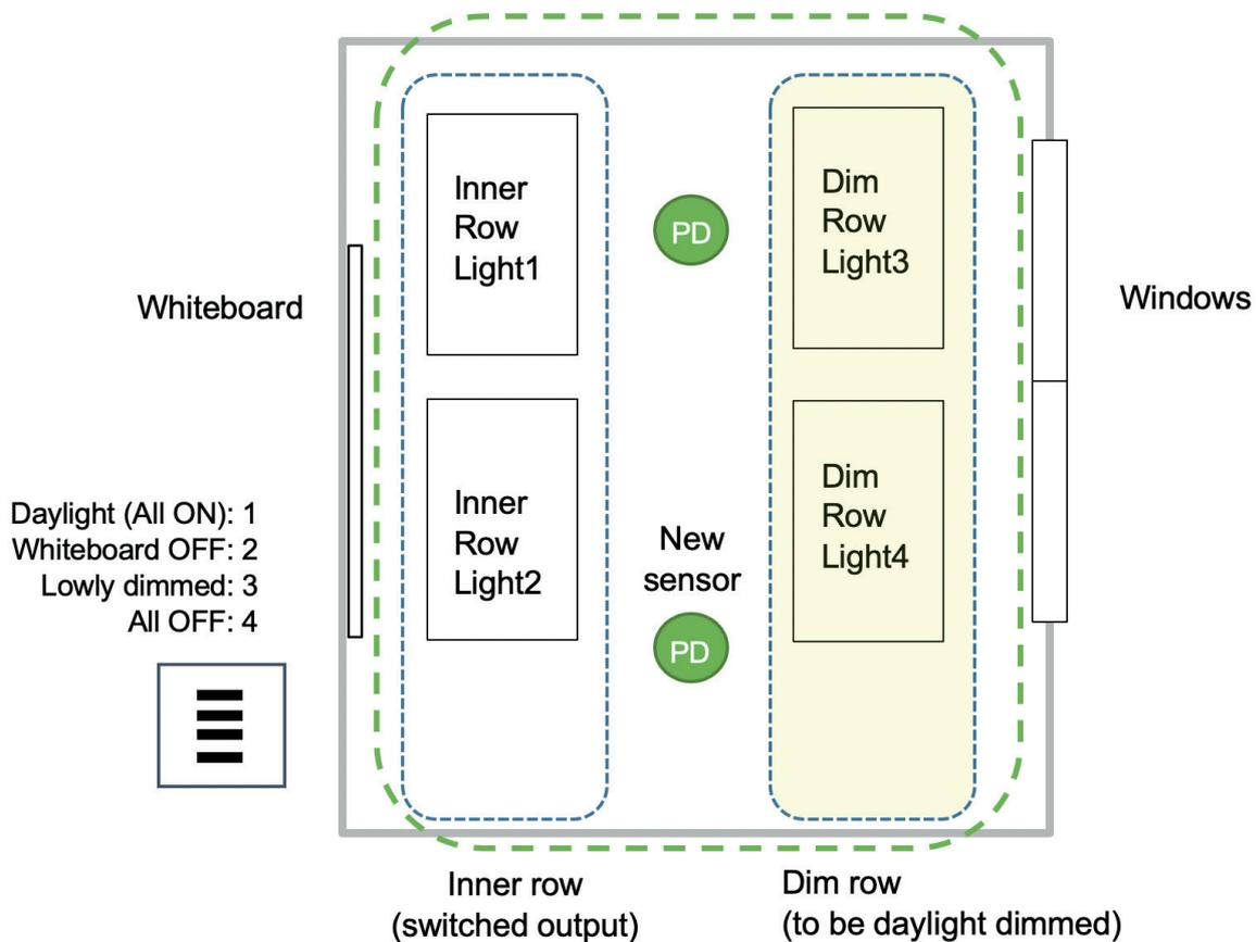
Additional occupancy sensors to control the same group of lights as the first sensor can be added by pairing the new sensor to the same network and setting its occupancy parameters to control the same ON and OFF scenes as that of the first occupancy sensor.
