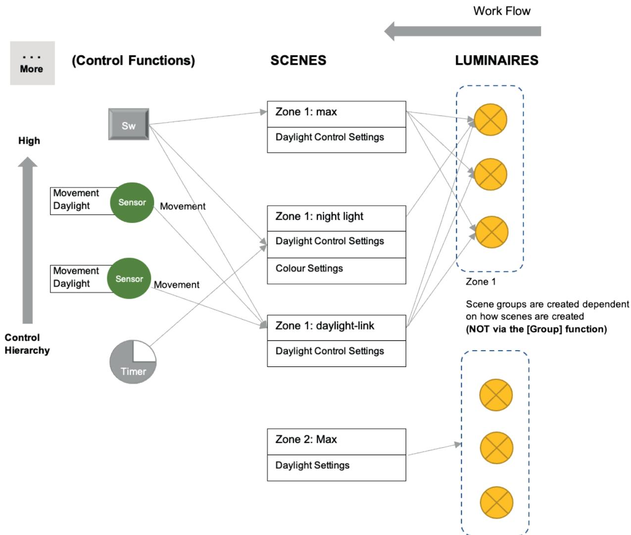
Each light fixture is grouped to act with the same behaviour using **scenes**. Control functions, such as occupancy control, then call these scenes to activate them. The **luminaire groups cannot** be used in conjunction with these scenes and they are primarily for manual group switch and dim operation on the app only.
