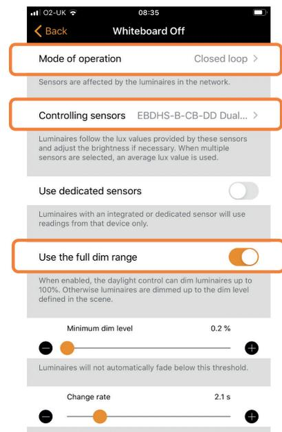
All the luminaires within this scene will now be under the control of the daylight control function. Allow a minute or so for it to take effect. The default settings will give a slow but smooth non-distracting response.
