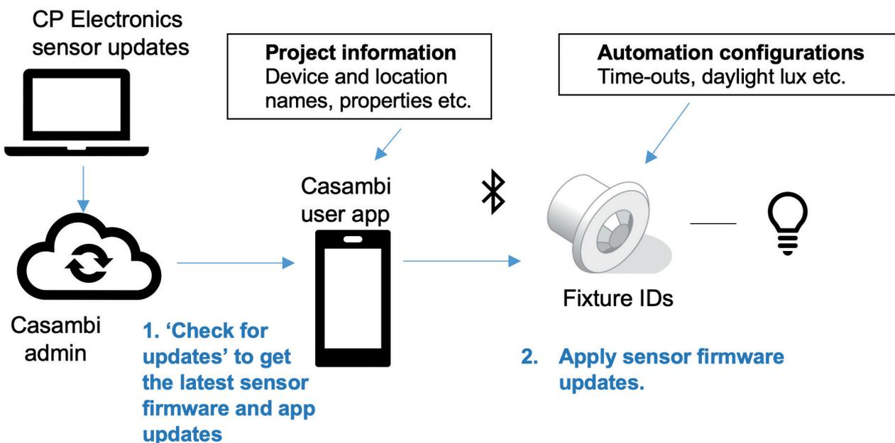
Different models of CP Electronics Casambi sensors will have different **fixture IDs** for example EBDHS-B-CB-DD for a high bay sensor or EBDSPiR-CB-DD for a standard ceiling sensor.
