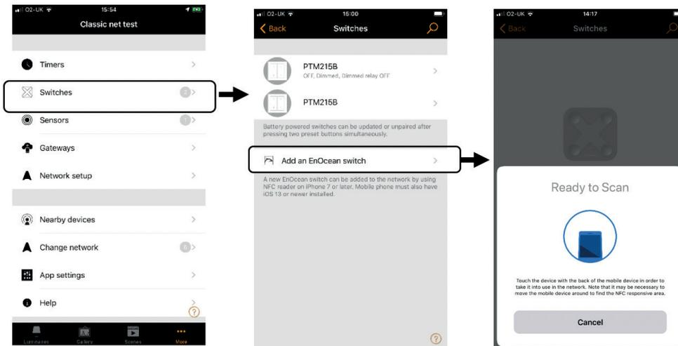
Place the top end of the phone near to the EnOcean switch and make a tap action for best response.
