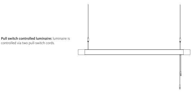
One for brightness control and on/off and the other one for colour temperature control and on/off.
