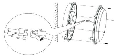
**5**: Connect the DC plugs, put back the cover to the back plate and fix it by the screws.
