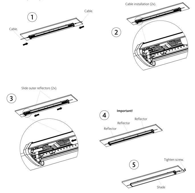
Internal through-wiring (pre-installed).
