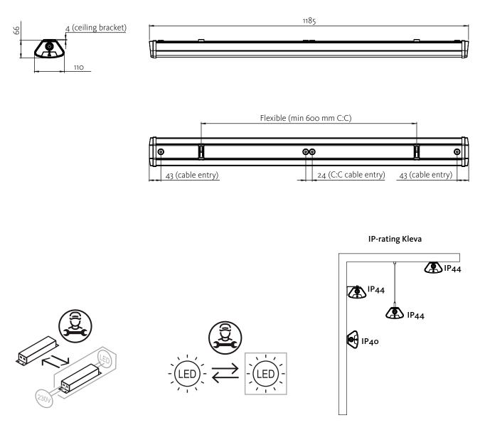
The luminaire contains a control gear and a replaceable LED light source that shall only be replaced by manufacturer.
