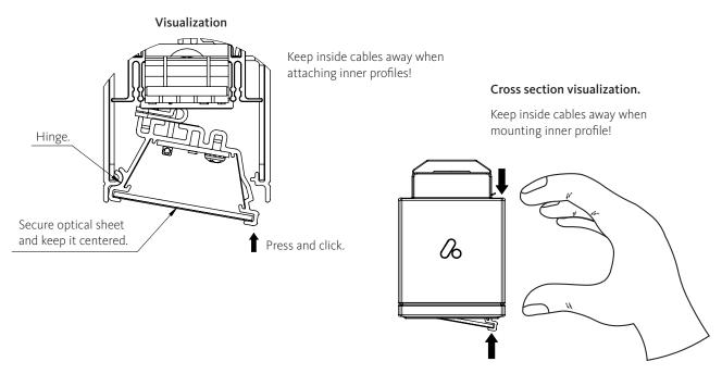
**6**: After installation; move optics to centre, without any light gaps. Place "light traps" at each end. Applicable for opal and microprismatic versions.
