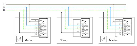
1: L-out for powering on/off luminaires. Max 400 W total power.
